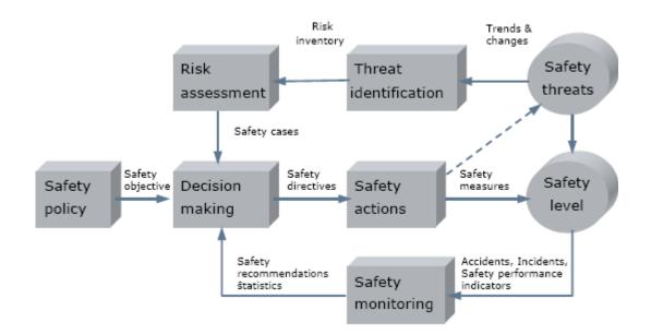
Figure 13: The safety management process (from DETEC, the National Aerospace Laboratory NLR and Van der Geest et al., 2003)
